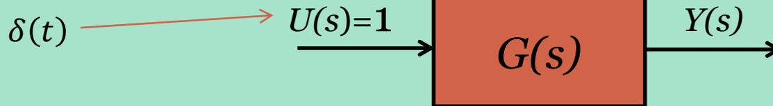
$$\text{sen } \omega t \xrightarrow{\text{Laplace}} \frac{\omega}{s^2 + \omega^2} = \frac{Y(s)}{U(s)} = G(s)$$
