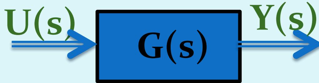
$$\mathbf{G}(s) = \left[ \begin{array}{c|c} A & B \\ \hline C & D \end{array} \right]$$
