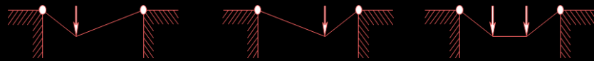
(b) A 'flexible' structure, such as a cable, can change drastically its shape, when loading varies
