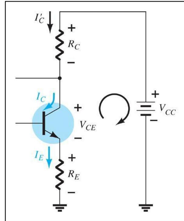
**Exemplo 1**Determine  $V_{CEQ}$  e  $I_{EQ}$  para o circuito abaixo.
