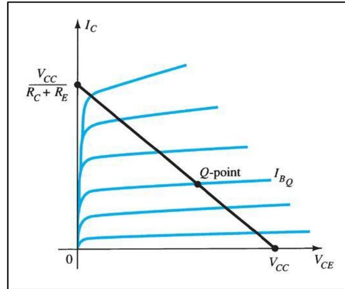
The endpoints can be determined from the load line.
