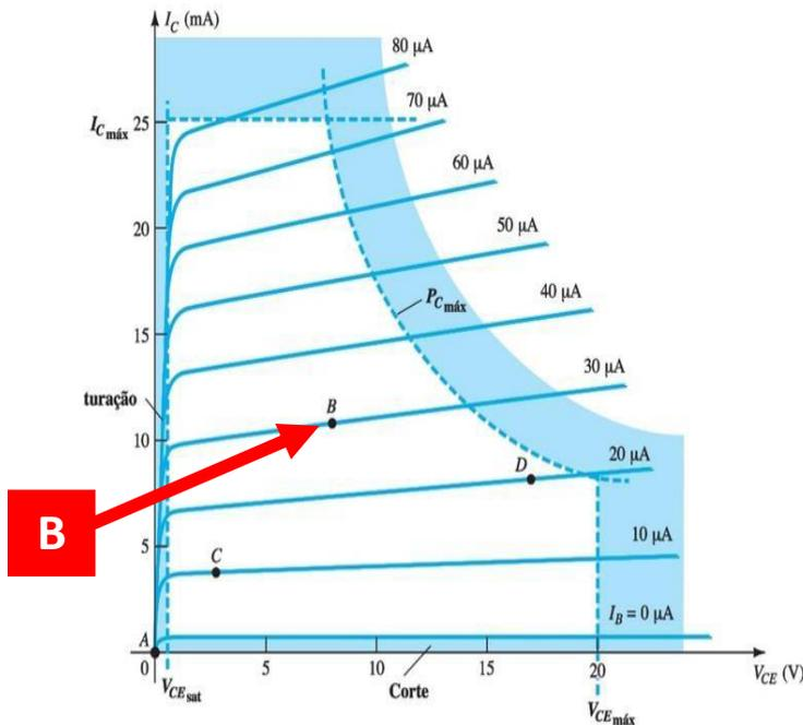
The small signal model accounts for the behavior which is linear around an operating point. When the large signal is in amplitude say more than 1/5 of  $V_{CC}$ , a rule of thumb, the behavior becomes non linear and we have to use the model which accounts for non-linearity, and thus called large signal model.
