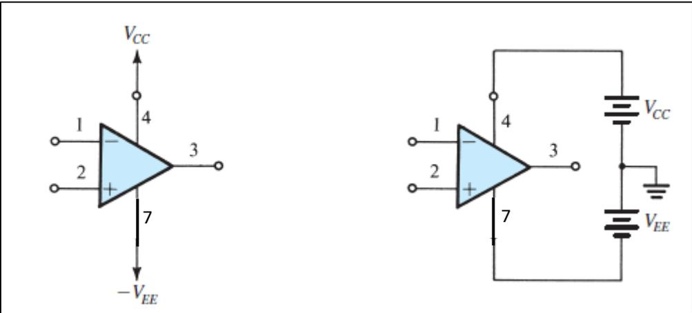
The op amp shown is connected to dc power supplies !
