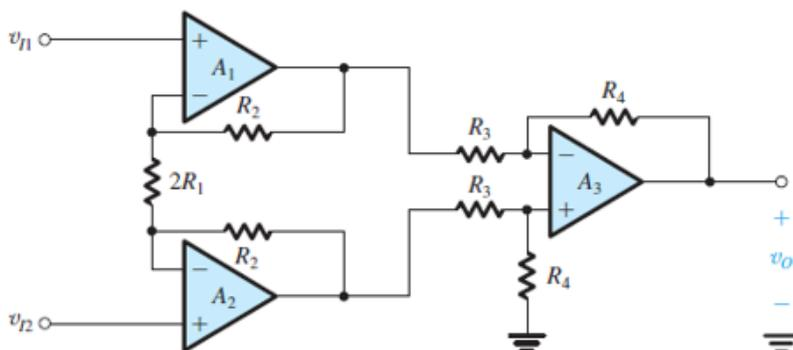
$$v_o = \frac{R_4}{R_3} \left( 1 + \frac{2R_2}{2R_1} \right) v_{Id}$$
