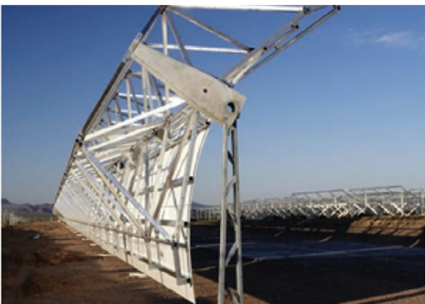
Figure 20: Solargenix / Gossamer Spaceframes / Acciona aluminum space frame parabolic trough collector at Nevada Solar One site (south of Las Vegas, NV) [12]
