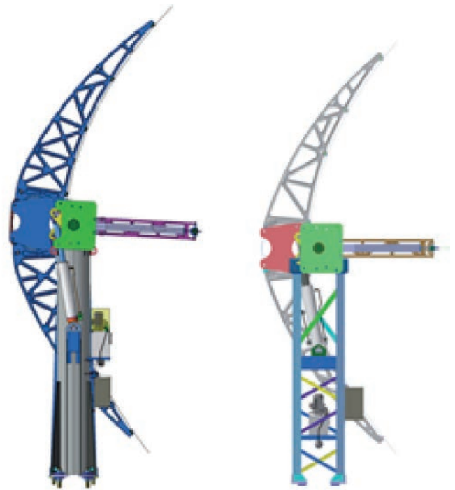
Figure 30: Sener_2 collector (left) and Sener 1 collector (right)
