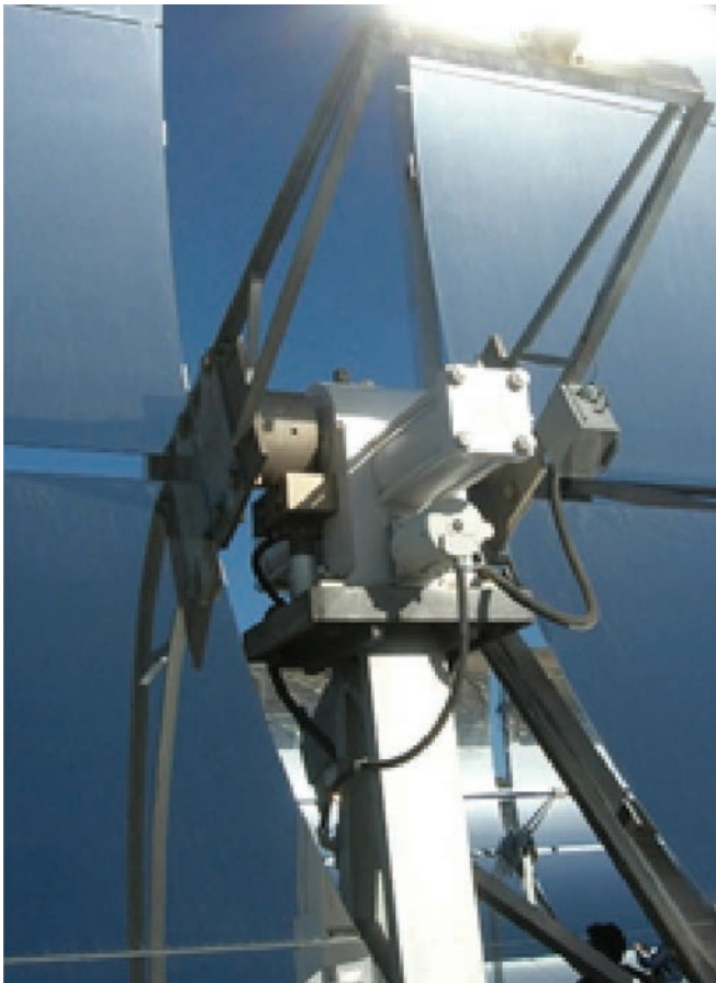
Figure 52: SGX-2 (Nevada Solar One) drive
