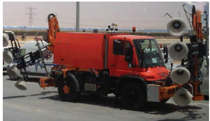
Figure 57: Cleaning vehicle at Shams power plant (Abu Dhabi)
