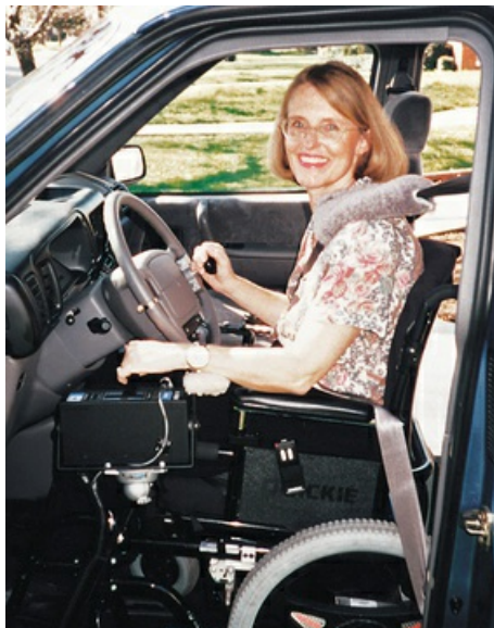
FIG 11.19 This client was experiencing difficulties driving and at work because progression of her multiple sclerosis exceeded the activity demands of pushing a manual wheelchair. Driving from a power wheelchair and using an electronic gas-brake hand control decreased the activity demands on her upper extremities, enabling her to drive safely and work full time as a teacher.
