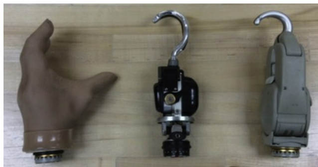
FIG 43.13 Examples of electrically powered prehensor terminal devices. Left , System Electric Hand (Ottobock). Center , Electric Terminal Device (Motion Control, Inc.). Right , System Electric Greifer (Ottobock).
