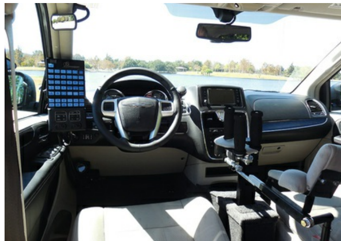
FIG 11.29 Some people with severe disabilities are able to drive if matched with the right technology. This variation of the Scott Driving system allows the steering, gas, and brake to be operated with a single arm. (Courtesy Driving Systems, Van Nuys, CA.)
