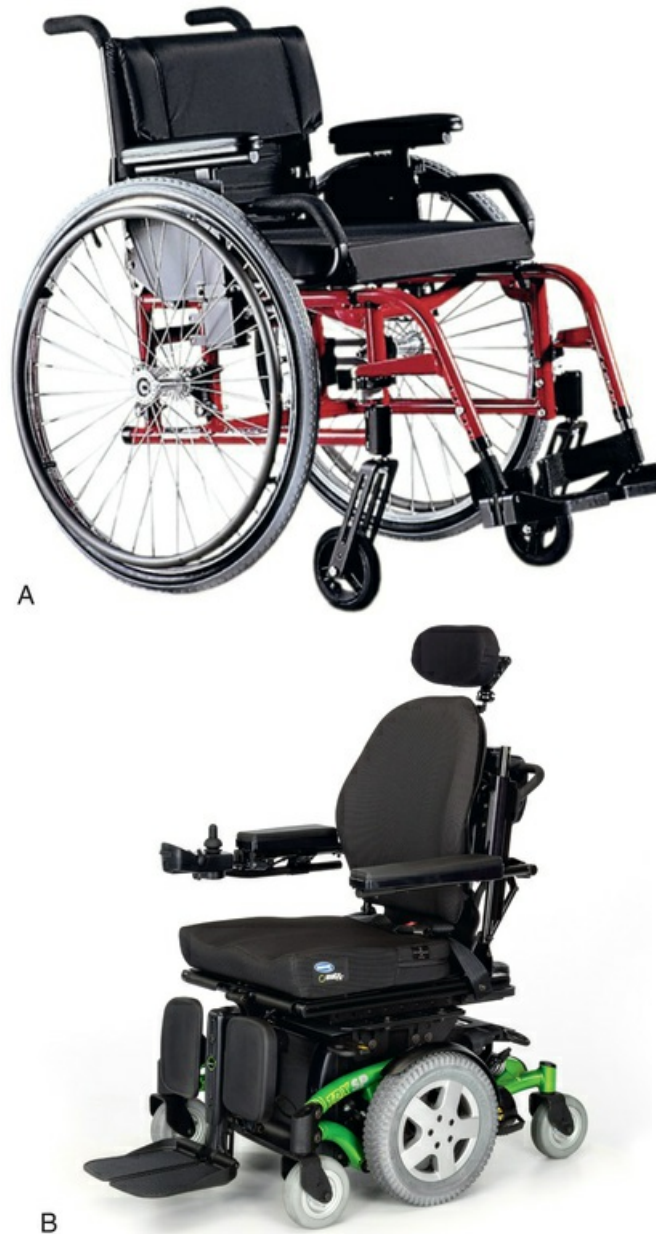
FIG 11.3 Manual vs. electric wheelchair. A, Rigid-frame chair with swing-away footrests. B, Power-driven wheelchair with hand control. (A, Courtesy Quickie Designs, Phoenix, AZ; B, Courtesy Invacare, Elyria, OH.)
