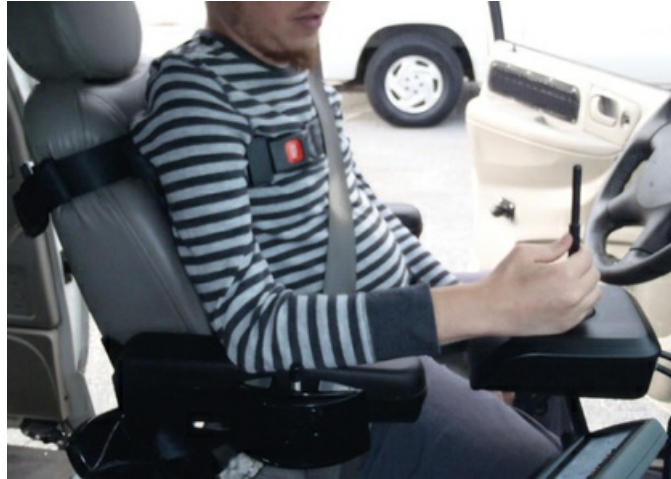
FIG 11.25 This client with muscular dystrophy required a joystick system to operate the primary controls for driving. Evaluations and training requirements for clients using high-tech systems are more complicated and time intensive.
