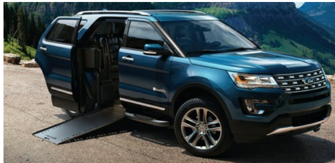
FIG 11.27 The BraunAbility MXV is a wheelchair-accessible SUV that might be an appropriate alternative to a minivan for some clients. (Courtesy Braun, Winamac, IN.)
