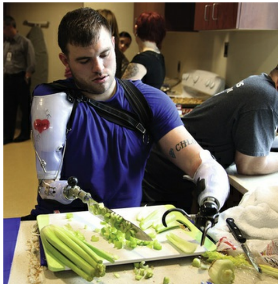
FIG 43.23 Individual with bilateral upper limb loss using a combination of prosthetic systems. On the right side he is using a transhumeral body-powered system with an activity-specific terminal device. On the left side he is using a transradial myoelectric system with an electric hook.
