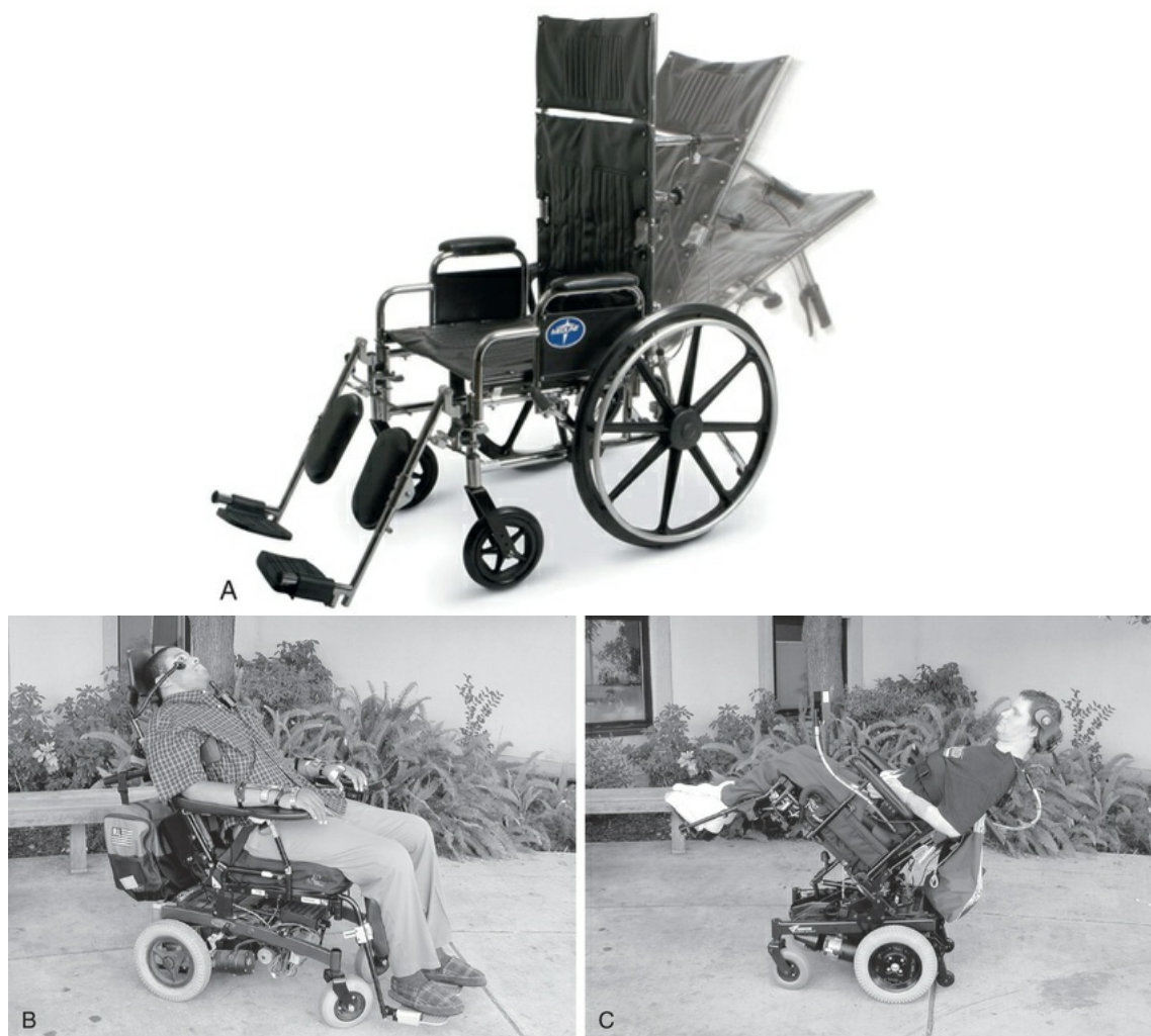
FIG 11.4 Manual recline vs. power recline wheelchair. A, Reclining back on folding frame. B, Low-shear power recline with collar mount chin control on electric wheelchair. C, Tilt system with head control on electric wheelchair. (A, Courtesy Medline Industries, Inc., 2016; B and C, Courtesy Luis Gonzalez.)
