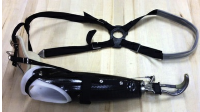
FIG 43.9 Transradial body-powered prosthesis with a one-cable design and figure-eight harness.
