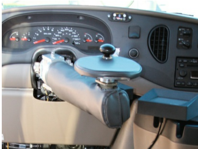
FIG 11.24 A steering wheel that can be placed in a horizontal position can enable steering for clients who lack upward range to reach a traditional wheel. (Courtesy Drive-Master, Fairfield, NJ.)
