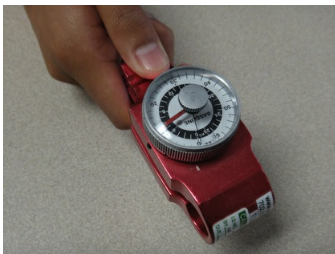
FIG 39.3 A pinch gauge is used to evaluate pinch strength in a variety of prehension patterns of pinch.
