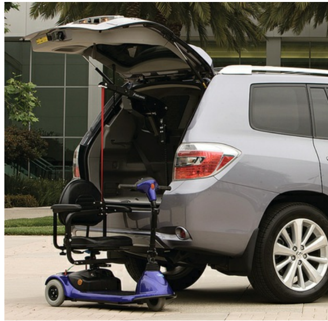
FIG 11.26 Bruno's Curb-Sider lifts and stows a scooter or power wheelchair inside a minivan by the push of a button on a handheld pendant. (Courtesy Bruno Independent Living Aids, Oconomowoc, WI.)
