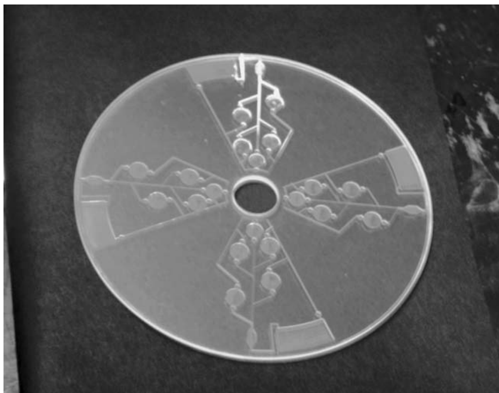
FIGURE 4.33 CNC-machined plastic lab CD platform. (Courtesy of Drs. Madou and Lee, OSU.)
