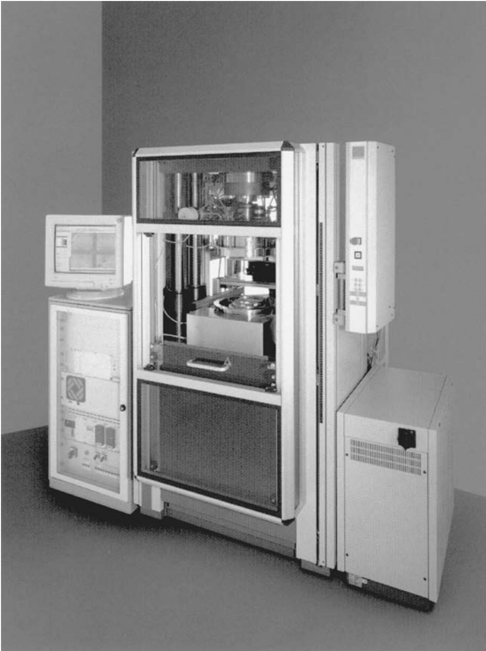
FIGURE 4.47 JENOPTIK HEX 03 hot embossing system manufactured by Jenoptik Mikrotechnik, GmbH.
