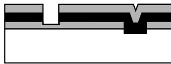
FIGURE 3.101 Masking and process sequence preparing a wafer for laterally grown porous polysilicon. (Reprinted with permission from Field, L. [1987] “Low-Stress Nitrides for Use in Electronic Devices,” in EECS/ERL Res. Summary , University of California, Berkeley pp. 42–43.)
