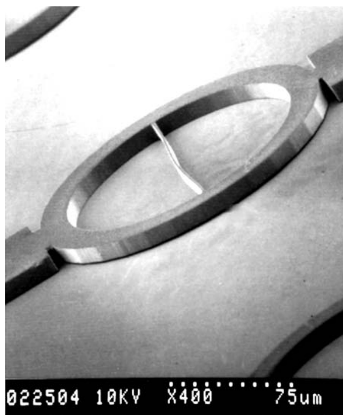
FIGURE 5.15 DXRL patterned and electroformed nickel ring and beam structure used to measure tensile internal strain via mechanical buckling. The beam cross member 2 \mu\text{m} wide and 18 \mu\text{m} thick was originally straight after electroforming and has now buckled after release via a sacrificial etch as a result of tensile internal strain. Together with the outer and inner ring radii of 100 \mu\text{m} and 80 \mu\text{m} , respectively, the critical buckling geometry of this structure represents a 0.08% internal tensile strain.
