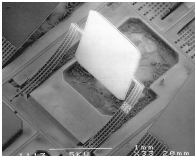
FIGURE 3.47 Optical filter of porous Si. SEM of a free-standing porous Si microplate containing a multilayered optical interference filter. The wavelength can be tuned by tilting the microplate, using the integrated thermal bimorph microactuator. The tilt angle is a function of the actuator DC voltage. This filter element can be used to build a microspectrometer. (Courtesy of Dr. Gerhard Lammel, EPFL, Lausanne, Switzerland.)
