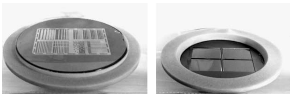
FIGURE 5.6 Frontside (left) and backside view of 1- \mu\text{m} thick silicon nitride membrane X-ray mask 5 \times 7 cm in area supported by a 4" diameter silicon wafer with 8- \mu\text{m} thick patterned and electroplated gold absorber layer.
