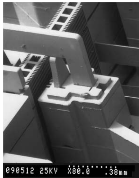
FIGURE 5.41 Five-layer stacked 78 permalloy linear actuator mechanism over 1 mm in height.
