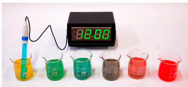
Figure 2. Setup of a demonstration pH meter with LED display of pH values.
