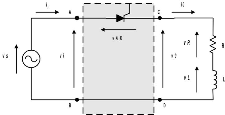
$$i_N = \text{sen}(\omega.t - \phi) - e^{(\alpha - \omega.t)/\tan\phi} \cdot \text{sen}(\alpha - \phi)$$
