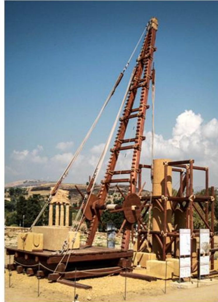
Re-creation of Greek mēchanē (crane) found at Valley of the Temples, Agrigento, Sicily. Photo: T. Hines 2019
