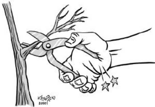
Poorly-designed tool: Handle presses into base of palm and requires user to open after each cut (no spring).
