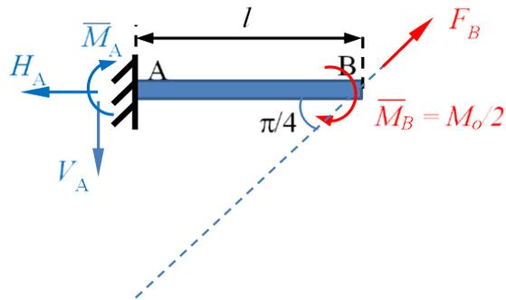
$$\theta_B = \frac{\partial U^*}{\partial \bar{M}_B} = \int_0^l \frac{M}{EI} \frac{\partial M}{\partial \bar{M}_B} dx$$
