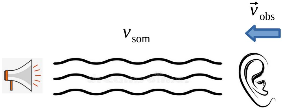
$$f_{\text{obs}} = f_{\text{fonte}} \frac{v_{\text{som}} + v_{\text{obs}}}{v_{\text{som}}}$$
