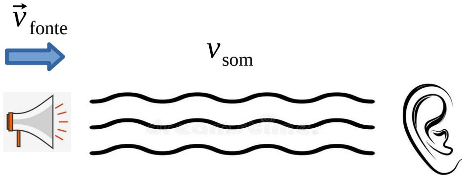
$$f_{\text{obs}} = f_{\text{fonte}} \frac{v_{\text{som}}}{v_{\text{som}} - v_{\text{fonte}}}$$
