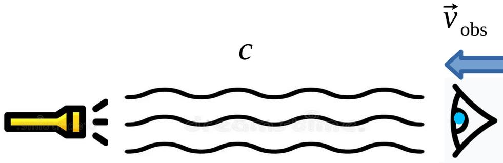
$$f_{\text{obs}} = f_{\text{fonte}} \gamma \frac{c + v_{\text{obs}}}{c}$$
