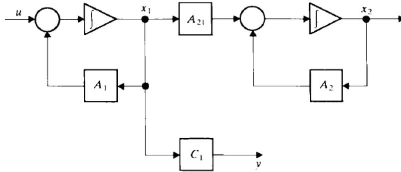
Figure 5.9 Systems in tandem that are unobservable.
