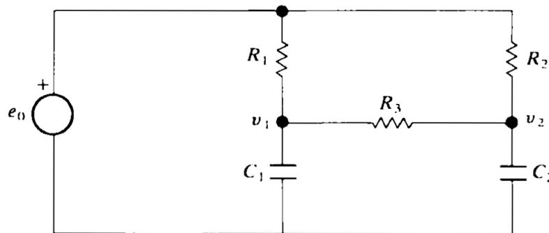
Figure 5.5 Electrical bridge network.
