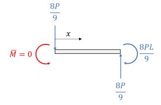
$$\theta = \frac{\partial U^*}{\partial \overline{M}} = \frac{1}{EI} \int_0^L M(x) \frac{\partial M}{\partial \overline{M}} dx$$
