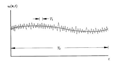
$$\begin{aligned} u_i'(\mathbf{x}) = & \lim_{T \to \infty} \frac{1}{T} \int_t^{t+T} u_i'(\mathbf{x}, t) dt = \lim_{T \to \infty} \frac{1}{T} \int_t^{t+T} [u_i(\mathbf{x}, t) - U_i(\mathbf{x})] dt = \\ & \lim_{T \to \infty} \frac{1}{T} \int_t^{t+T} [u_i(\mathbf{x}, t)] dt - \lim_{T \to \infty} \frac{1}{T} \int_t^{t+T} [U_i(\mathbf{x})] dt = 0 \end{aligned}$$
