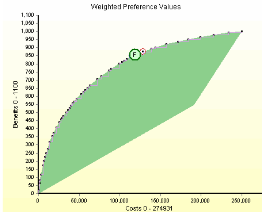
Figure 3: An efficient frontier created from an MCDA model. The graph displays cumulative benefits versus cumulative costs. Each point represents another project, with the F position defining the affordable portfolio: all projects down and to the left of F are within the available budget.
