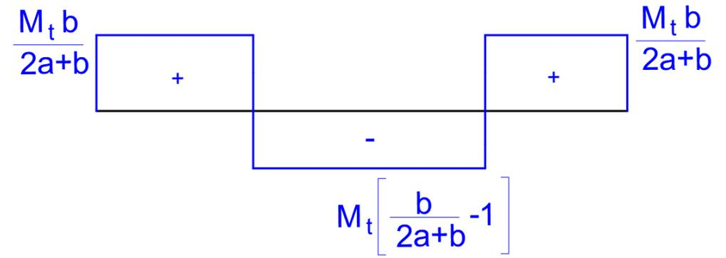
Trecho AB e CD:  $\tau_{AB} = \frac{T_{AB}}{J} \rho_{max} = \frac{M_t \cdot b}{(2a + b)} \frac{\rho_{max}}{J}$
