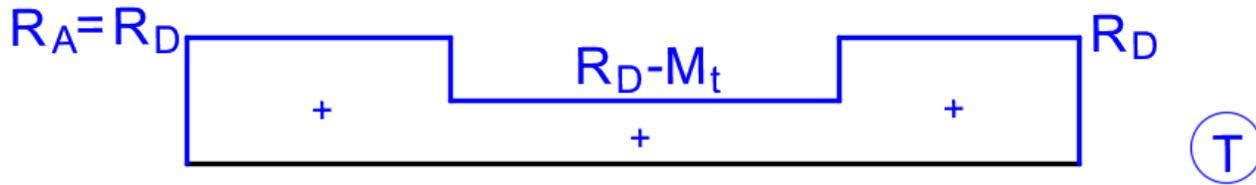
$$\phi_D = \phi_A + \left( \frac{T.L}{G.I_p} \right)_{AB \rightarrow CD} = 0 + \frac{R_D \cdot a}{GJ} + \frac{(R_D - M_t) \cdot b}{GJ} + \frac{R_D \cdot a}{GJ} = 0 \rightarrow R_D = \frac{M_t \cdot b}{2a + b}$$
