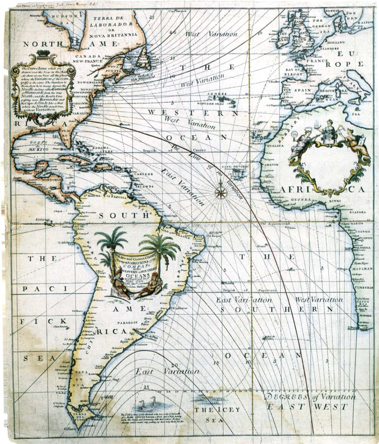
Figure 1.2 Map by Edmund Halley, 1701, produced using data collected during two voyages on the Paramore (sometimes spelt Paramour ), 1698–1700. The curved lines are isogons showing the angle between magnetic and true (or geographic) north. Source: N. J. W. Thrower (1972) Maps and Man , Prentice-Hall.
