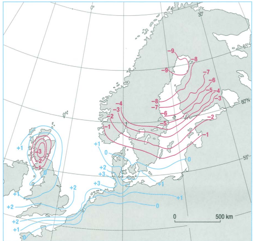
Figure 6.10 The present annual rate of change in sea-level in north-western Europe. The contours represent rises (positive) or falls (negative) in mm per year.
