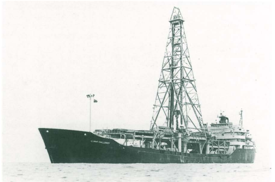
Figure 1.20 Glomar Challenger . Thrusters in the bow and stern were controlled by computer to maintain station within 30 m of a point directly above an acoustic beacon on the ocean floor. Drilling could thus proceed without snapping the drill string.
