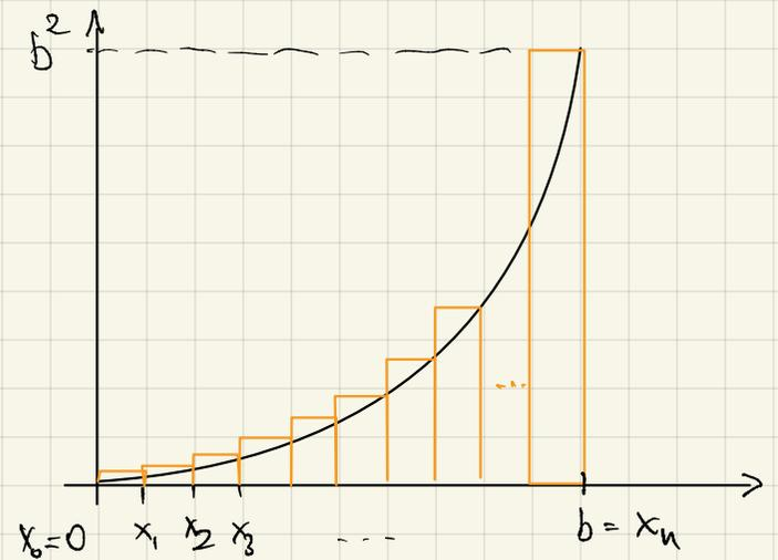
$$S_n = \frac{b}{n} \left[ \left(\frac{b}{n}\right)^2 + \left(\frac{2b}{n}\right)^2 + \dots + \left(\frac{nb}{n}\right)^2 \right]$$
