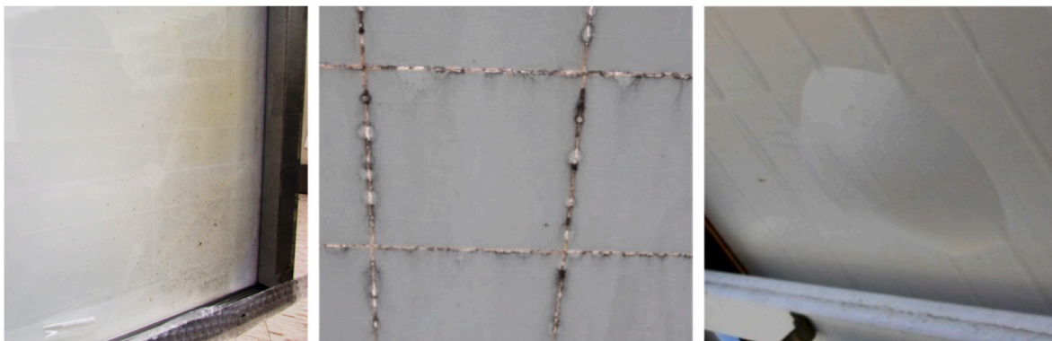
Fig. 6. Examples of backsheet degradation and failure: discolouration (left), cracking (center), and delamination (right). Reproduced with permission from Refs. [25,99].
