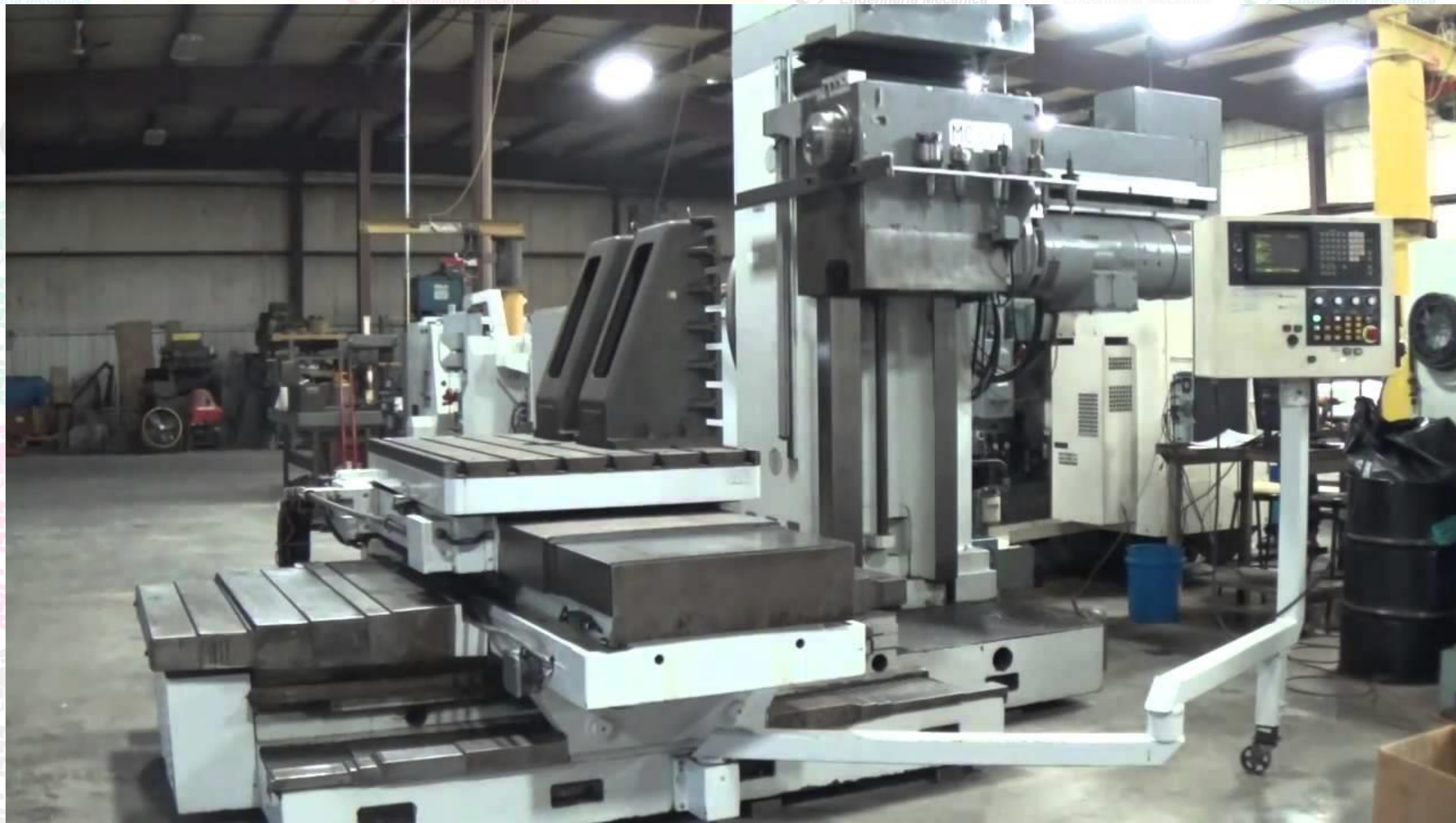
Alesa Monti MCS100 5-Axis CNC Horizontal Boring Mill '80s/'90s
