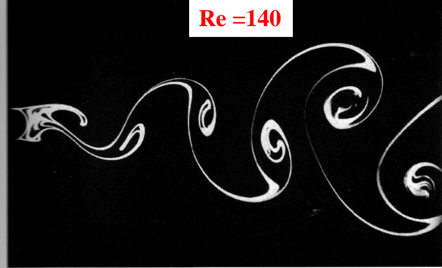
Fig. 1.6. Kármán vortex street behind a circular cylinder at R = 140 (Van Dyke 1982). Photograph S. Taneda.
