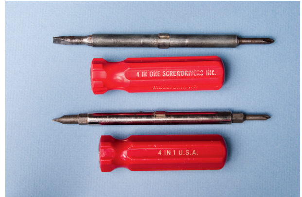
Figure 22-82 Revealing the inner parts of the two screwdrivers.
