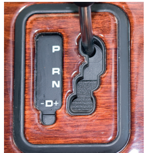
Figure 22-57 Shifting pattern in Mercedes-Benz Sprinter, even better at helping prevent physical overshoot.
