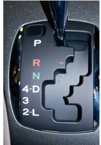
Figure 22-56 Shifting pattern in Toyota Sienna van, helping prevent physical overshoot.
