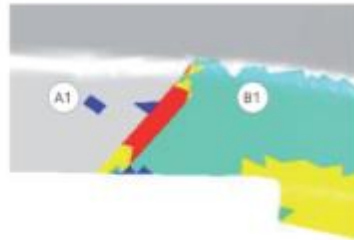
Tailored Blanks FLC allows to predict rupture by stamping simulation
