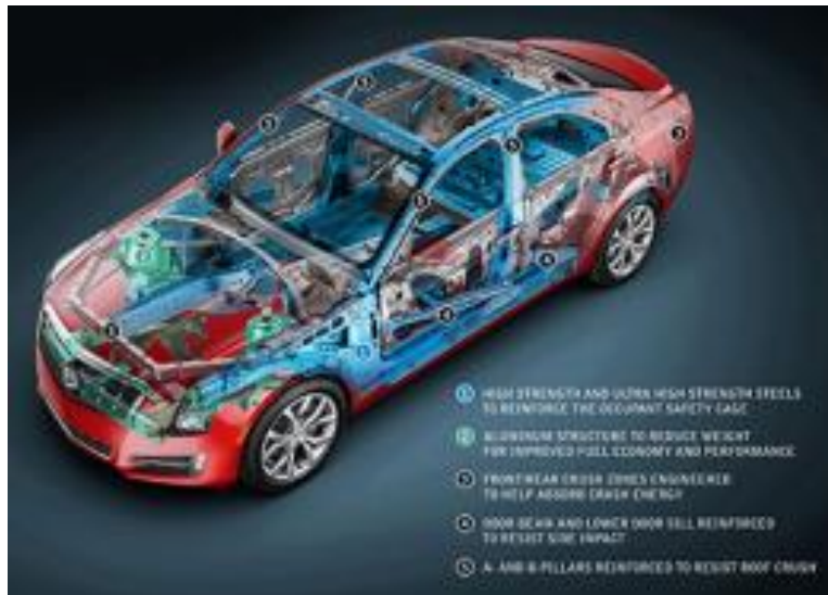
AHSS as well as aluminum are used in the body structure of the 2013 Cadillac ATS.
