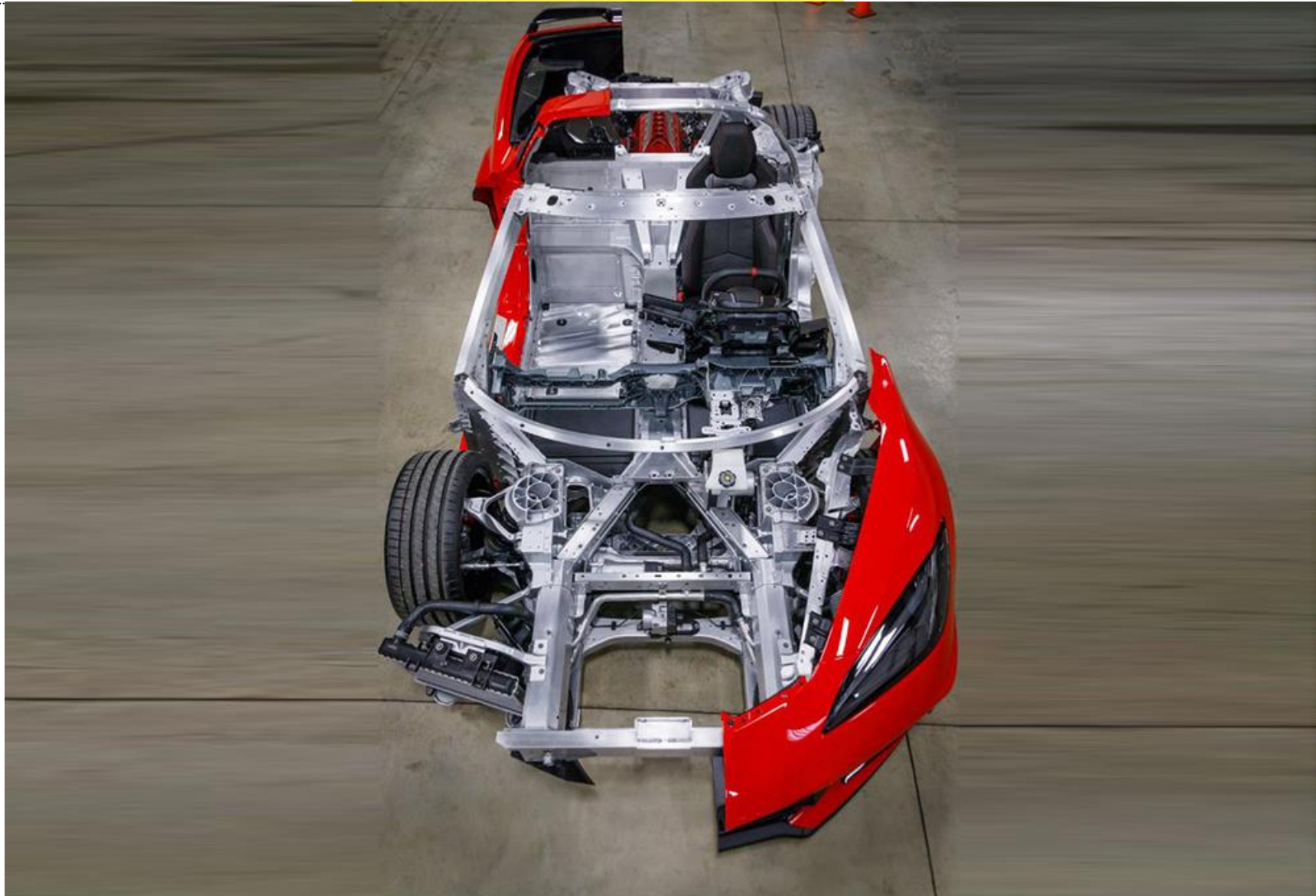
Corvette's new aluminum-intensive space frame laid bare. (GM)
