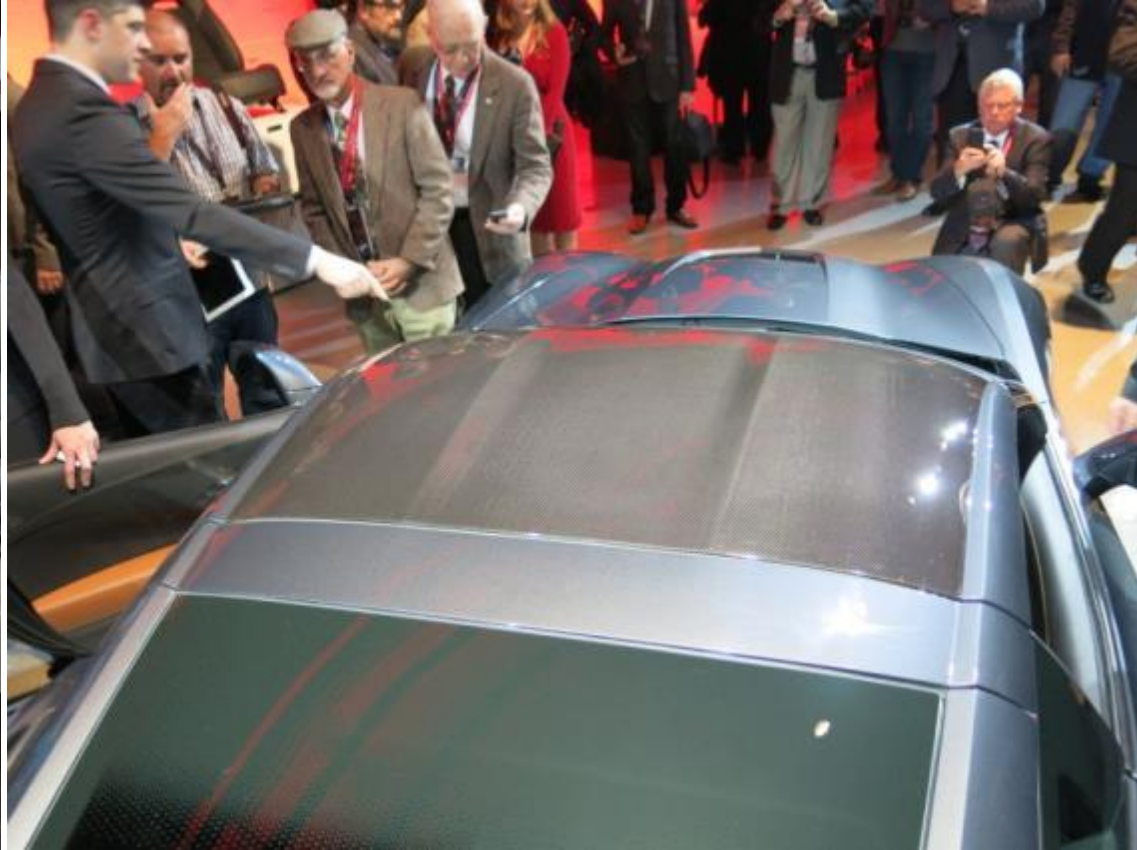
Carbon-fiber roof panel and hood are molded by Plasan Carbon Composites in western Michigan.
