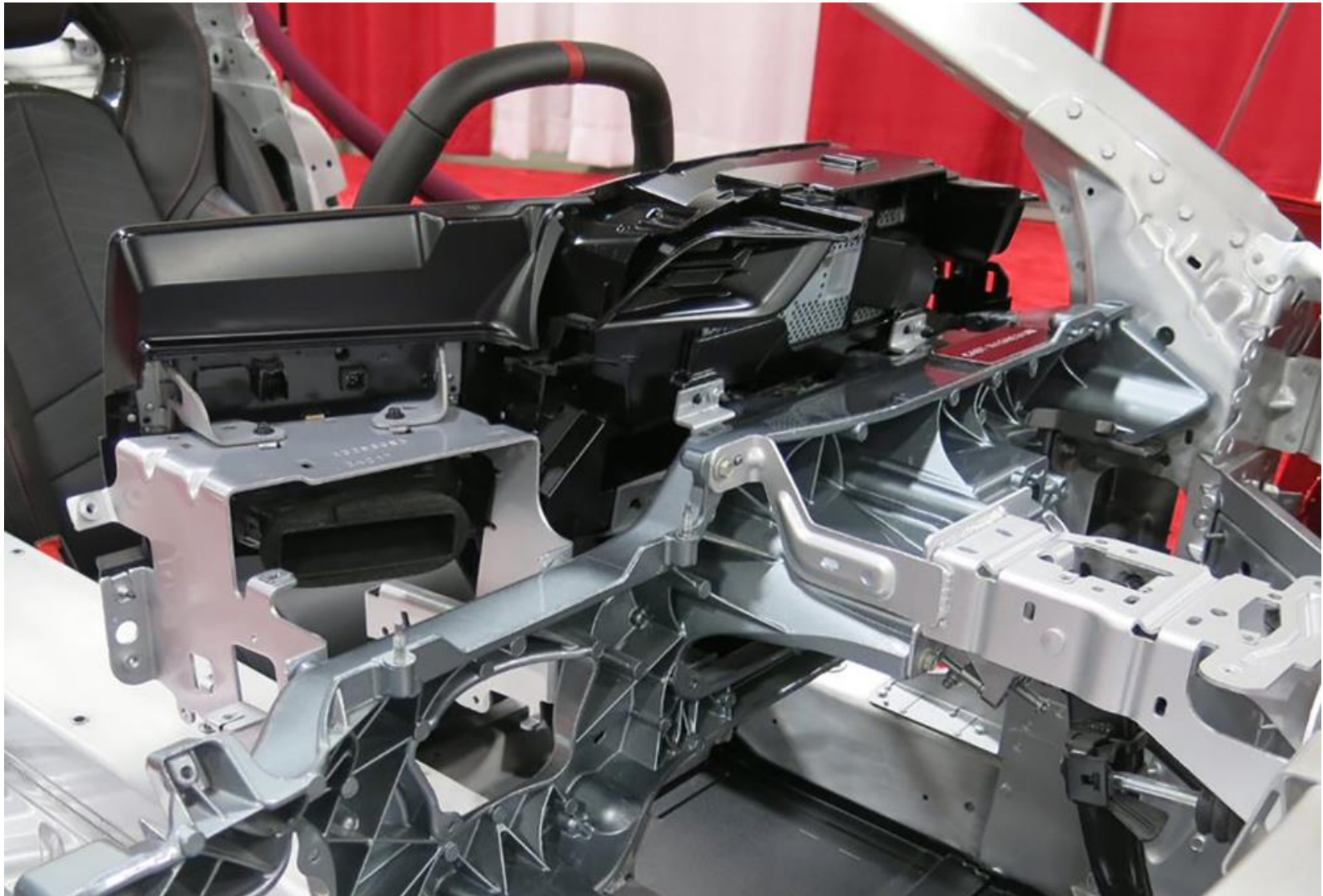
Details of C8's magnesium crosscar beam and instrument module. At left is deep-section center-tunnel structure. (SAE/Lindsay Brooke)
