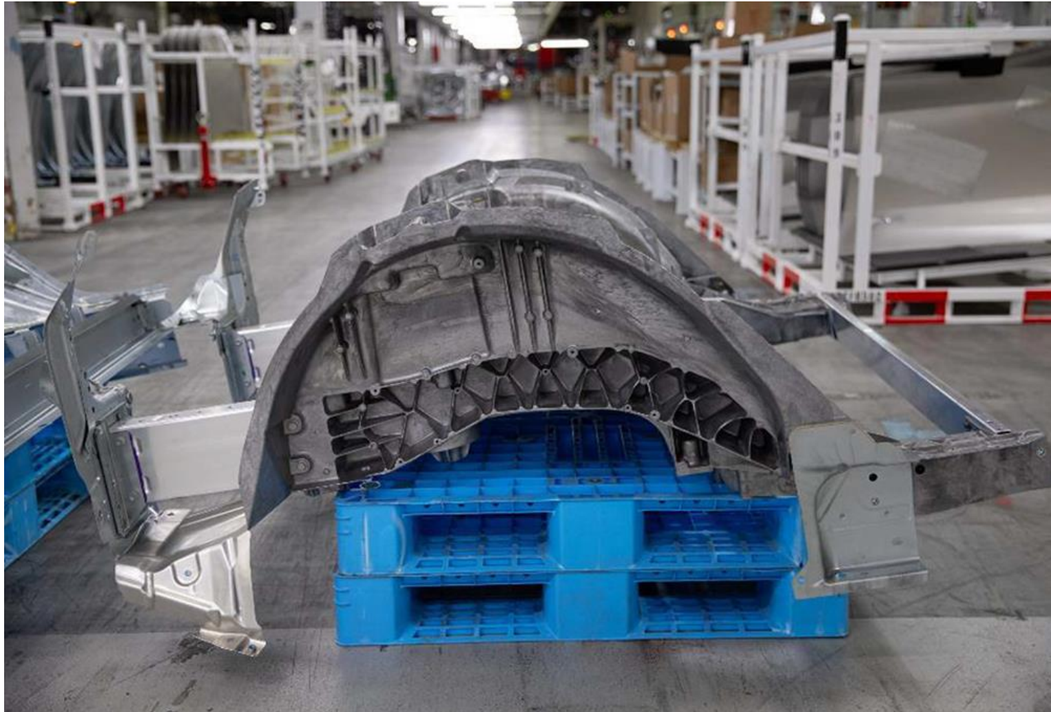
One side of the current Model Y's two-piece rear-underbody aluminum casting. (Tesla)
