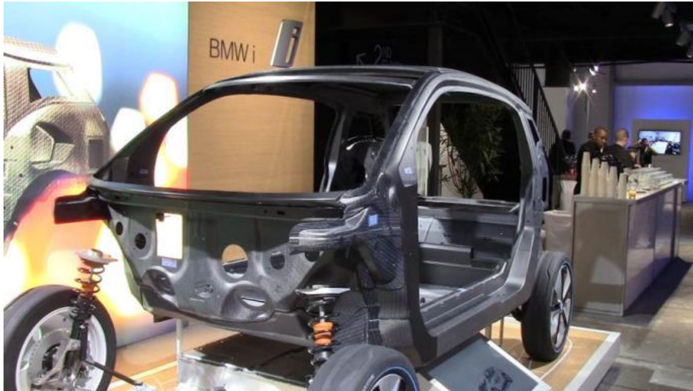
The bodies of BMW's i brand models will use carbon-fiber-reinforced plastic.
