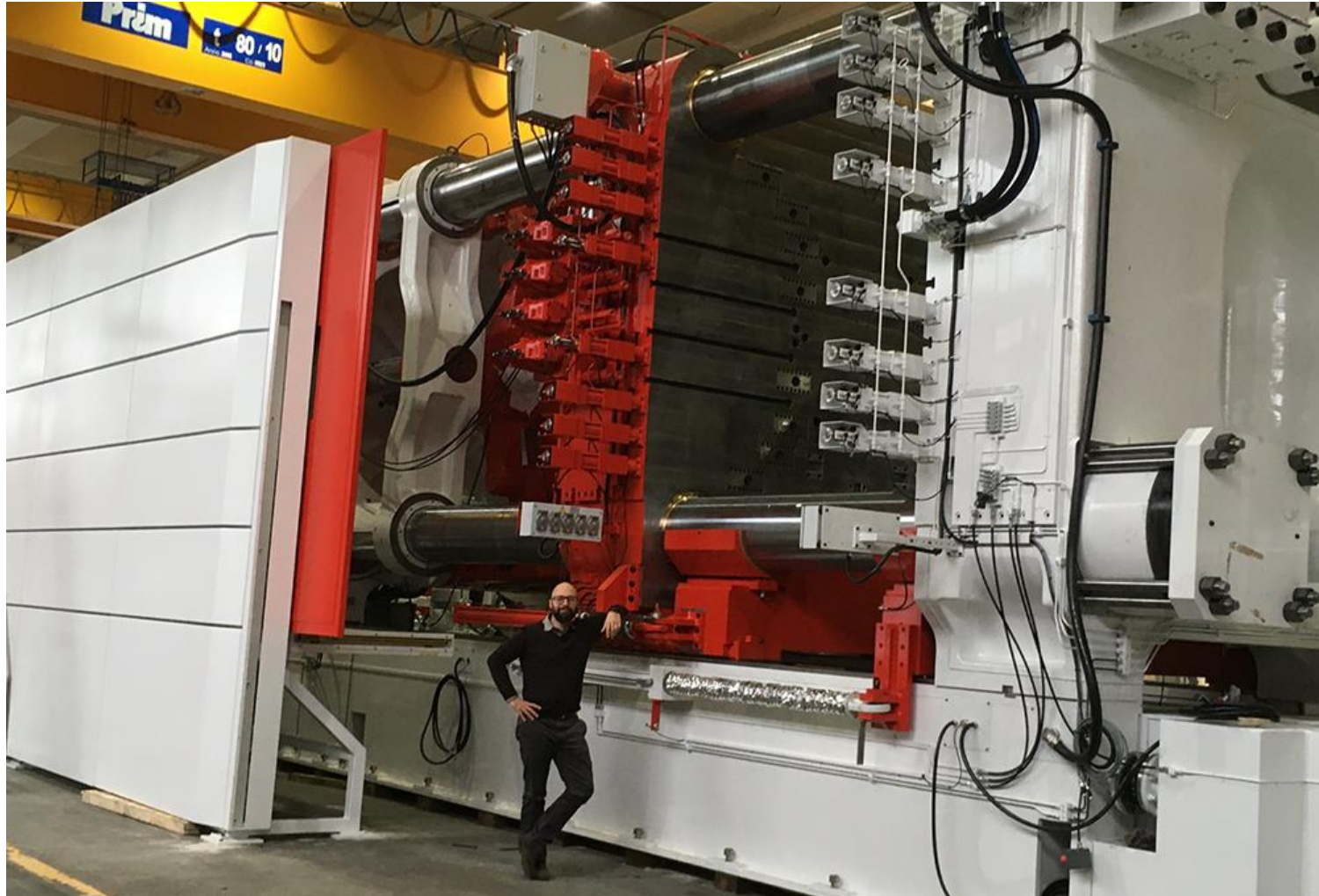
IDRA Group's OL 5500 CS, part of the company's new Giga Press lineup designed to produce large aluminum die castings. (IDRA Group)
