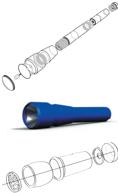
Fig. 5 The flashlight sketch represents a quick view exploded along a single axis while the CAD rendering uses photorealism to show the assembly including the battery. (TEAMS Design, Chicago.)
