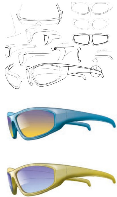
Fig. 18 This sequence moves from loose sketches to a single concept to be rendered in multiple ways.
