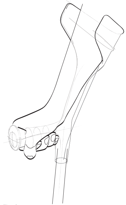
Fig. 2 This perspective sketch of a crutch includes a hand and arm to provide context. The ghosted-in centerline helps reinforce the main axes.
