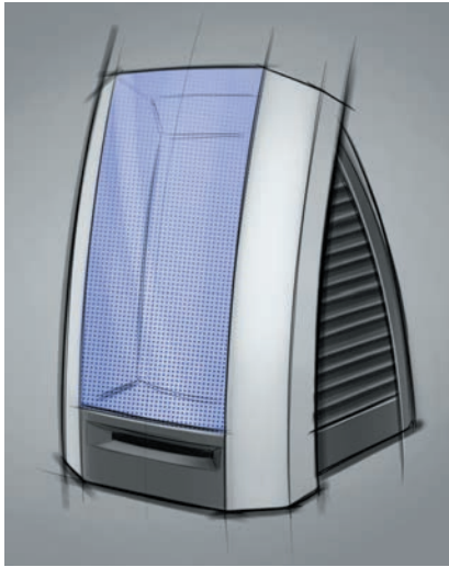
Fig. 22 In this perspective sketch the arcs extend beyond the form as part of the dynamic sketching process but also as a way to emphasize the dominant curves that define the form. (TEAMS Design, Chicago.)
