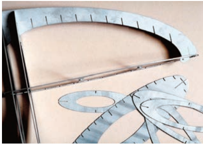
Fig. 15 A close-up detail of the elliptical sections machined and slotted out of aluminum sheet.
