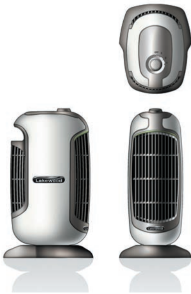
Fig. 20 These renderings from Radius Design (Chicago) demonstrate a photorealistic approach combined with the accuracy of orthographic.
