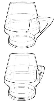
Fig. 3 Changing the vantage point (angle of view) so that the handle is clearly seen in relation to the body of the cup makes the sketch easier to read.
