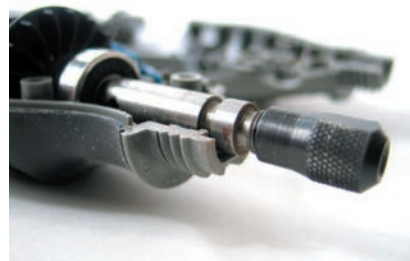
Fig. 10 This sketch shows an exploded view of a handheld grinder concept. The two halves have been split at the parting line, thus revealing some of the internal components. Separate parts like buttons, insert panels or electronic components can be revealed in this way.
