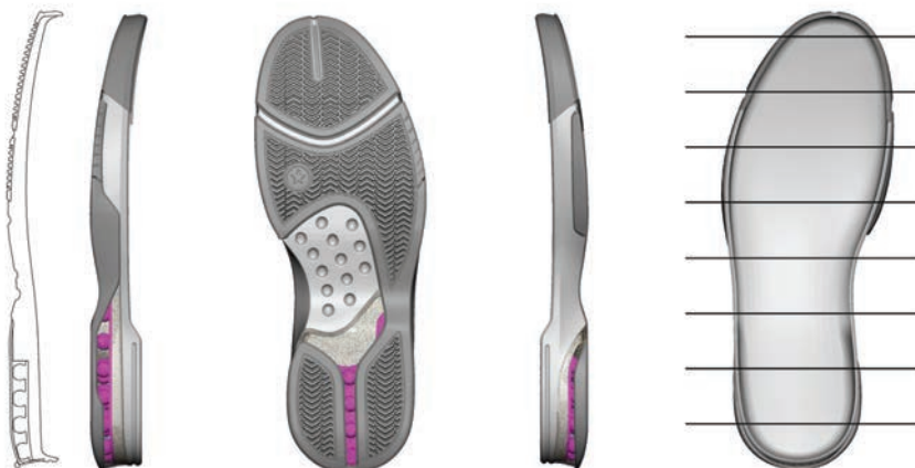
Fig. 39 This shoe concept for Converse shows a top view sectioned in eight places that correspond to the various section cuts above. Sections are an ideal way to understand geometry at a particular point in space.
