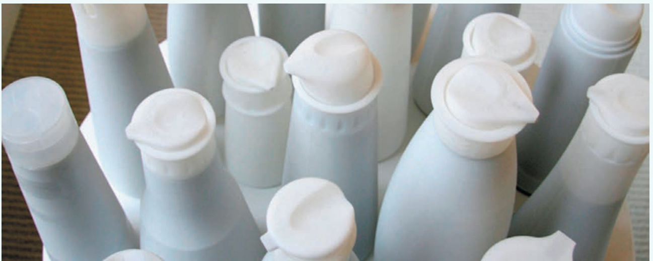
These 3D printed prototypes are dramatically lit for a line review after they have been cleaned up and painted.
