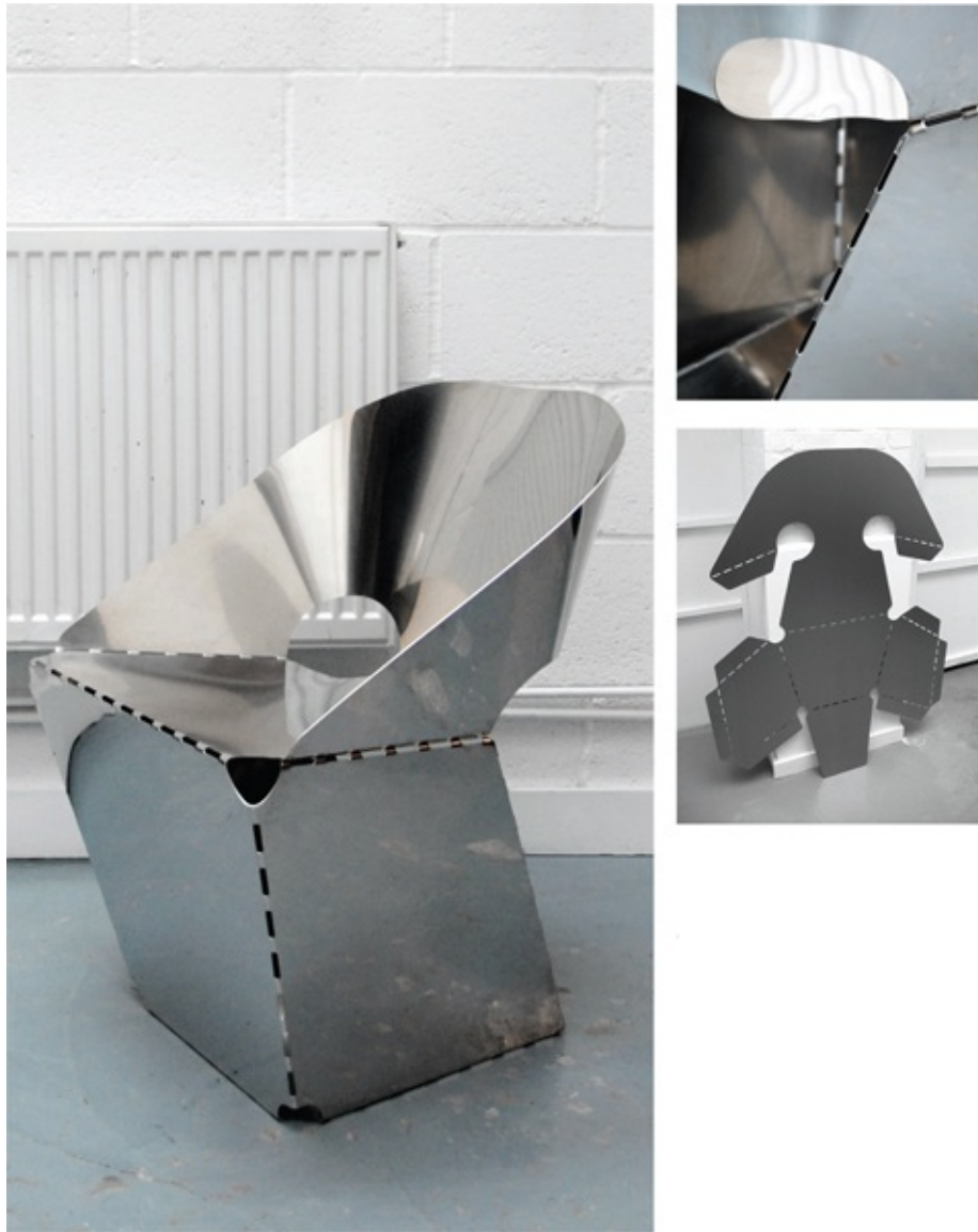
Sheet Steel chair, designed and produced by Max Lamb, 2008. First, it is formed from a single sheet of steel (above), then bent along the punched holes for assembly (top and left).
