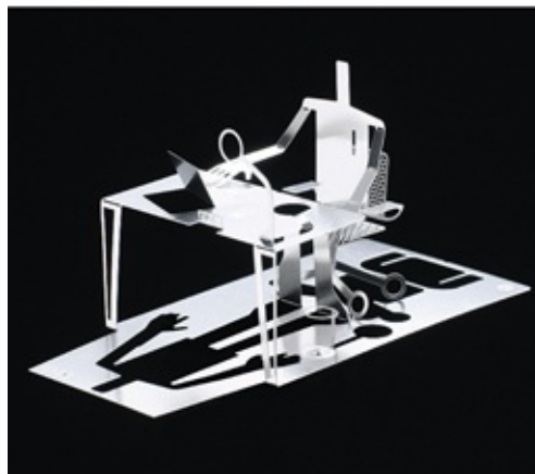
Micro World, designed by Sam Buxton, 2003. This is part of a series of fold-up metal sculpture business cards, where each scene folds from a flat sheet of photo-etched stainless steel just 0.005in (0.15mm) thick. All are packaged flat with folding instructions for buyers to complete the sculpture.
