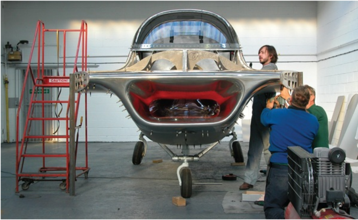
Kelvin 40 concept Jet, designed by Marc Newson, 2004. The partially riveted, welded, and bonded structure is shown (above), while (below) the designer completes his final check on the canopy latch system.
