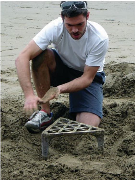
Pewter Stool, designed and made by Max Lamb, 2006. Cast into crude sand formations on a sandy beach, it takes shape as the incoming tide cools the molten metal.
