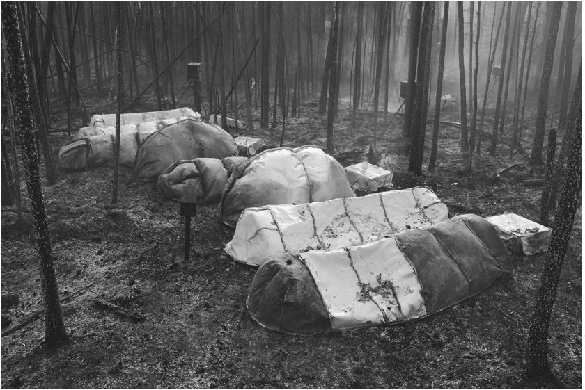
FIGURE 9.3. New-generation fire shelter test in Alberta, Canada: high temperatures melted the aluminum covering, exposing heat-resistant silica cloth (2015) (photo courtesy of Ian Grob/U.S. Forest Service).
