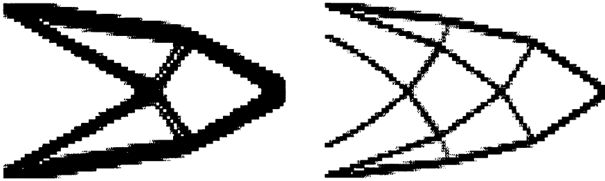
Figure 6.5.1 Optimal shapes for a fillet problem using microstructure.
