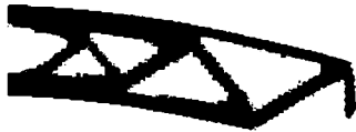
Fig. 2.11. Deformed configuration of the topology optimized for 144 kN (see Fig. 2.10). Note that the right-most bar supporting the load is un-bent in the deformed configuration (from Buhl et al. 2000).
