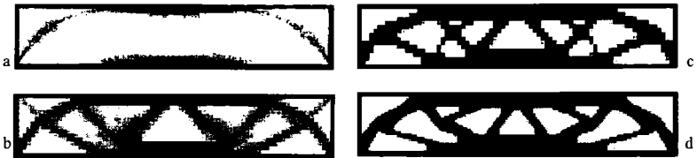
Fig. 3.6. Optimal design using a rank-2 material strain energy density with penalties on intermediate densities and on perimeter. a) shows the density distribution for the unpenalized case. In b) intermediate densities are penalized. In c) and d) intermediate densities and perimeter are penalized, with d) being a fine mesh variant of c) (from Jog et al. 1994).
