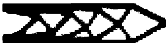
Fig. 2.13. Optimized topology for minimization of complementary elastic work (from Buhl et al. 2000).
