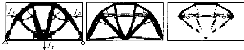
Fig. 3.25. Minimum compliance design. Left: In the absence of damage loads, Mid: With a constraint on the effect of damage loads, and Right: the distribution of damage in this optimal design (from Bendsøe & Díaz 1998).
