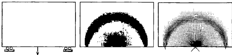
Fig. 3.10. Optimal design using an optimized rank-2 material strain energy density. Optimized designs computed using element wise constant density function and a 8-node displacement model. Center: the optimal density distribution, and Right: the associated principal stress distribution for a volume fraction of 20%. Note that grey area is not limited to biaxial response. The bicycle wheel like design has an area with radial uniaxial stress as well as a rim of circumferential uniaxial stress (the rim of a 'wheel') (from Jog et al. 1994).
