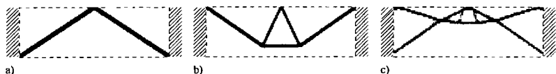
Fig. 2.16. Optimal topologies for the design problem in Figure 2.15. a) optimized topology for small displacement finite element modelling and b) optimized topology for large displacement modelling and c) optimized topology for large displacement modelling and two load-cases (from Buhl et al. 2000).
