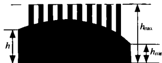
Fig. 3.20. Cross-section of the upper half of a rib-stiffened plate with one field of stiffeners running along the normal of the cutting plane.
