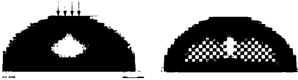
Fig. 3.5. Optimal design using a rank-2 material. Left: The optimal design using an element wise constant density function and a 8-node displacement model. Right: The unstable checkerboard solution obtained when using a 4-node displacement model (from Jog et al. 1994).
