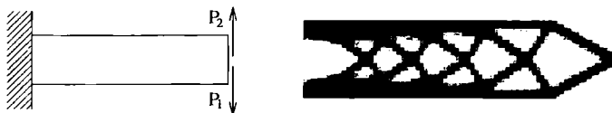
Fig. 2.12. A two-load case problem with two large loads acting in opposite vertical directions (from Buhl et al. 2000).
