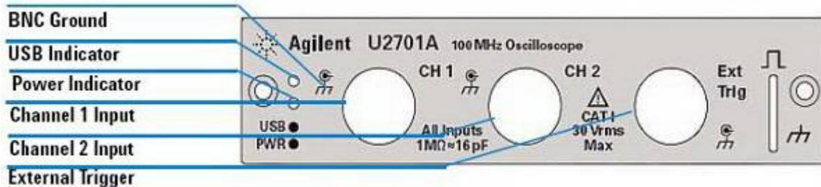
Figure C-1 – Front Panel of the U2701A
