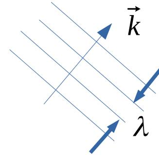
$$E(r, t) = \Re \left[ \underbrace{\frac{A_0}{r} e^{i(k \cdot r + \delta)}}_{Z_0(\vec{r})} e^{-i\omega t} \right]$$
