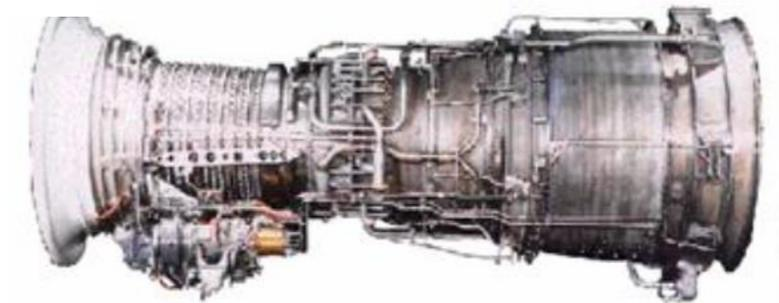
The LM2500 has four major components: a 16-stage, 18:1 pressure ratio compressor with seven stages of variable stators and inlet guide vanes; a fully annular combustor with externally mounted fuel nozzles; a two-stage, air-cooled high-pressure turbine which drives the compressor and the accessory-drive gearbox; and a six-stage, aerodynamically coupled, low-pressure power turbine which is driven by the gas generator's high-energy exhaust gas flow.
