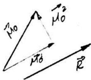
$$\vec{M}_O = \vec{M}_O^1 + \vec{M}_O^2 \quad \rightarrow \quad I = \vec{M}_O \cdot \vec{R} = \vec{M}_O^1 \cdot \vec{R} = \text{cte}$$
