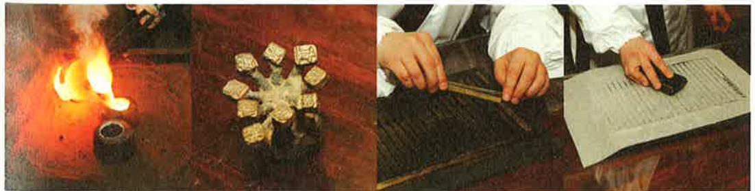
⑤ Pouring boiled iron ⑥ Completed metal types ⑦ Typesetting [composition, arrangement] ⑧ Printing
