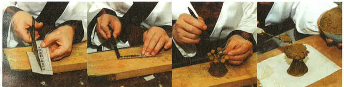
① Selecting the letter [character] model ② Pasting the model on a wooden block ③ Carving letters ④ Making a brass frame
