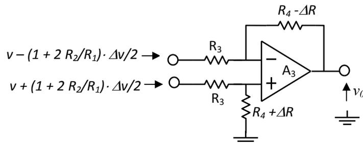
$$v_{01} = -\frac{(R_4 - \Delta R)}{R_3} \cdot (v - (1 + 2 R_2/R_1) \cdot \Delta v/2)$$
