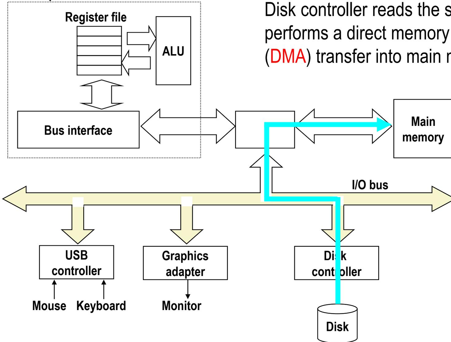
Disk controller reads the sector and performs a direct memory access (**DMA**) transfer into main memory.
