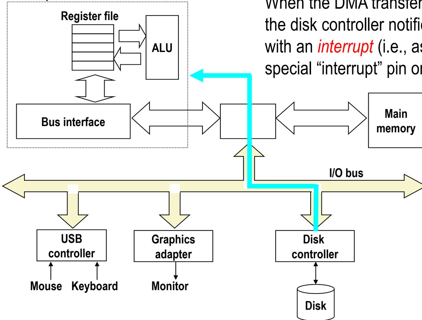
When the DMA transfer completes, the disk controller notifies the CPU with an *interrupt* (i.e., asserts a special “interrupt” pin on the CPU)
