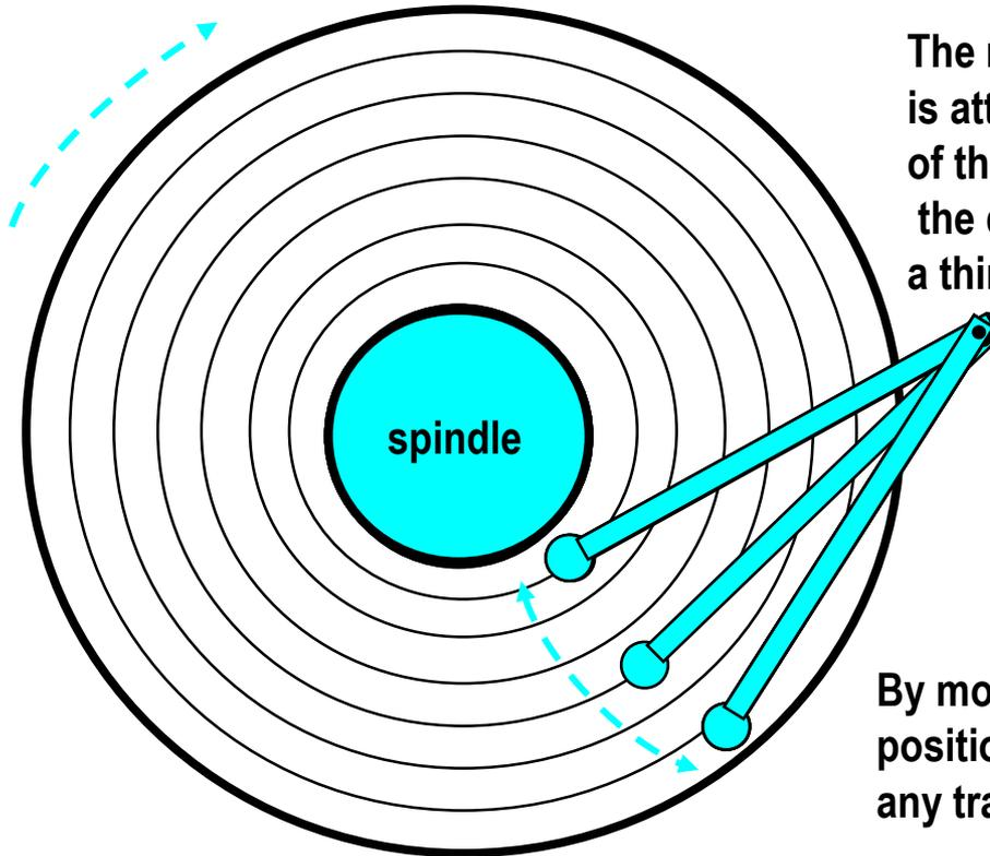
The read/write *head* is attached to the end of the *arm* and flies over the disk surface on a thin cushion of air.
