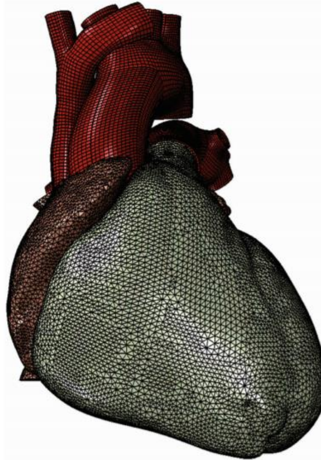
FIGURE 4. Mechanical finite element model of the human heart discretized with 449,560 linear tetrahedral elements, 12,915 linear quadrilateral shells, 7577 linear triangular shells, 636 linear truss elements, 16,824 rigid triangular elements, 130,290 nodes, and 443,564 mechanical degrees of freedom.
