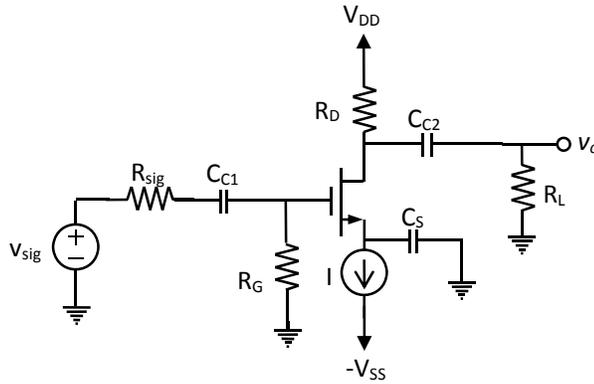
Respostas:  $A_M = -g_m R'_L \cdot \frac{R_G}{R_G + R_{sig}}$        $f_H = \frac{1}{2\pi(R_{sig} // R_G)[C_{gs} + C_{gd}(1 + g_m R'_L)]}$
