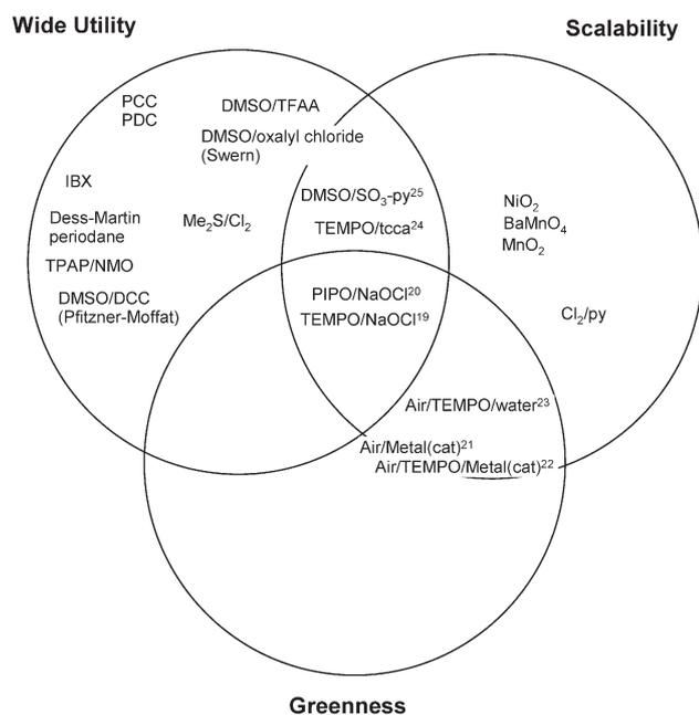
Fig. 3 Oxidation of primary alcohol to aldehyde.
