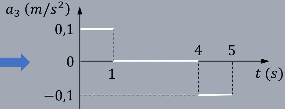
$$v_3 = -R_2\omega_2 \Rightarrow a_3 = -R_2\alpha_2 \Rightarrow \alpha_2 = -\frac{a_3}{R_2}$$
