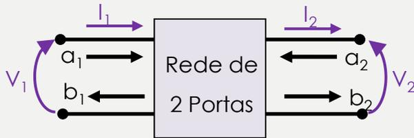
$$a_1 = \frac{V_1 + Z_0 I_1}{2\sqrt{Z_0}}; \quad b_1 = \frac{V_1 - Z_0 I_1}{2\sqrt{Z_0}}; \quad a_2 = \frac{V_2 - Z_0 I_2}{2\sqrt{Z_0}}; \quad b_2 = \frac{V_2 + Z_0 I_2}{2\sqrt{Z_0}}$$
