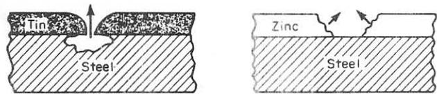
FIGURE 6 — Galvanic corrosion at perforation in tin and zinc-coated steel. Arrows indicate corrosive attack.
