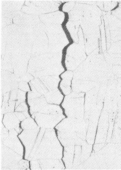
FIGURE 57 — Intergranular stress corrosion cracking of brass (E. N. Pugh).
