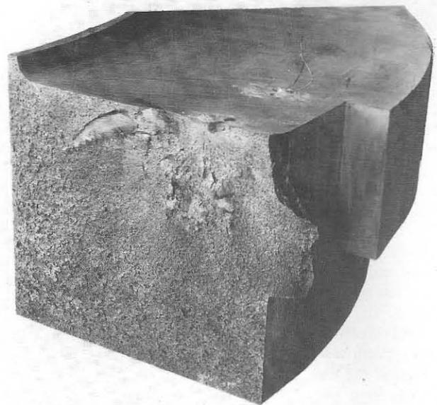
**FIGURE 43 – (Case B7) Fracture face (12 x 13 inches) of the extrusion chamber retaining ring. Fracture source markings are at one of the positions of thermocouple attachment by brazing; note a companion thermocouple.**
