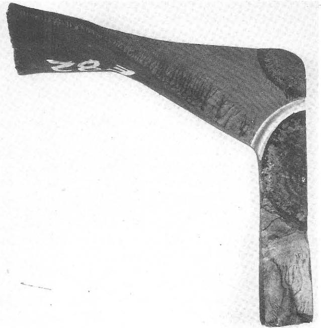
FIGURE 62 — (Case E4) Leakage region in the nozzle of the PVRC No. 4 vessel. The nozzle section was cooled with liquid nitrogen and split open in the plane of the two fatigue cracks (dark areas). The larger of the two fatigue cracks is noted to have penetrated through the thickness of the shell wall. The shiny arc between the cracks is a machine cut to remove a metal fin which covered a portion of the fatigue crack.
