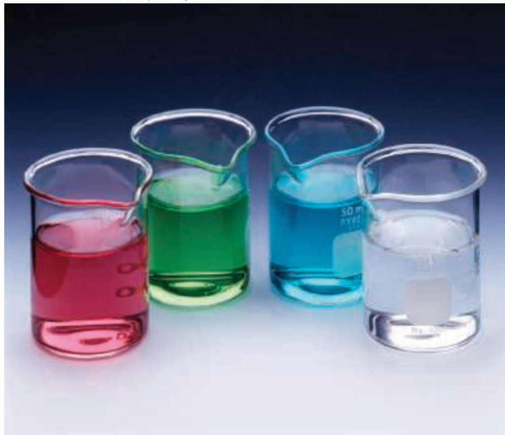
▲ Figure 23.4 Aqueous solutions of transition metal ions. Left to right: \text{Co}^{2+} , \text{Ni}^{2+} , \text{Cu}^{2+} , and \text{Zn}^{2+} . The counterion is nitrate in all cases.
