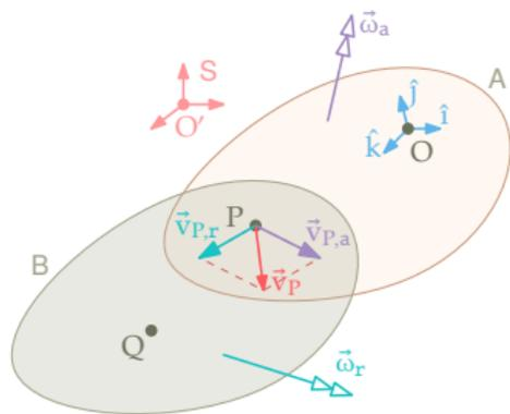
$$\vec{v}_P = \underbrace{\vec{v}_O + x \frac{d\hat{i}}{dt} + y \frac{d\hat{j}}{dt} + z \frac{d\hat{k}}{dt}}_{\vec{v}_{P,a}} + \underbrace{\dot{x}\hat{i} + \dot{y}\hat{j} + \dot{z}\hat{k}}_{\vec{v}_{P,r}}$$
