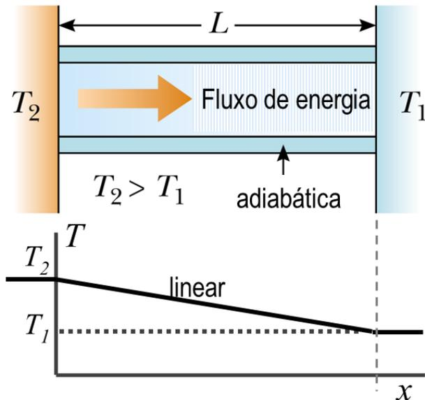
$$\frac{dT}{dx} = -\frac{T_2 - T_1}{L}$$
