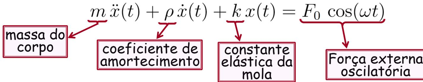
The diagram illustrates the equation of motion for a damped and forced harmonic oscillator. The equation is  $m \ddot{x}(t) + \rho \dot{x}(t) + k x(t) = F_0 \cos(\omega t)$ . Red arrows point from each term to a corresponding label in a box:  $m$  points to 'massa do corpo',  $\rho$  points to 'coeficiente de amortecimento',  $k$  points to 'constante elástica da mola', and  $F_0 \cos(\omega t)$  points to 'Força externa oscilatória'.
